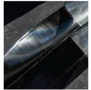
Clean, Uncontaminated Seams
